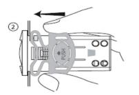
Slide the bracket to fix the device (step two)
