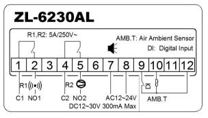
• Try with effort to layout the sensors and switches line apart from inductive load lines and power supply lines. The sensors and switches lines are not allowed go with the power supply lines and inductive load lines in a same
